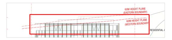
Figure 3: Extract of proposed Western Elevation, contravention of height standard shown in red (Source: UP Architects/Kann Finch)
