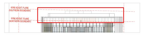
Figure 2 - Extract of proposed North Elevation, contravention of height standard shown in red (Source: UP Architects/Kann Finch)
